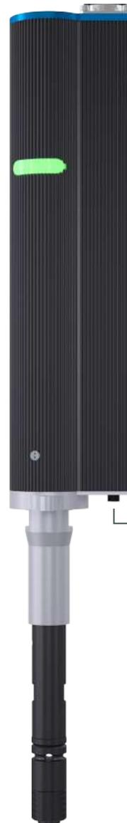
The illuminated field on the nutrunner indicates the status of the tightening process.
