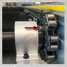
The correct functioning of the chains, heads and the conveyor is guaranteed by the torque limiter device installed on pinions that protect the conveyor in case of anomalies or chain blocks.
