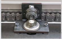
This smart device is appplied on transfer unit and gives the advantage to save a gearmotor for orthogonal transfer movement.
